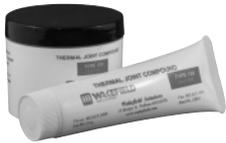
**120-\*) Thermal Compound** – The 120- Thermal Conducting Compound is a zinc oxide-filled, dielectric, silicone oil-based compound that facilitates heat transfer by filling voids and gaps between mating surfaces. The operating temperature range is -40° to 200°C (-40° to 392°F). It is available in a 5 oz tube or 2 & 8 oz jars.
