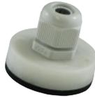
**DC-01) Duct collar** - The DC-01 is an adjustable collar for mounting the duct temperature sensor probes. It incorporates a foam backed mounting flange with 2 mounting holes. A compression type fitting accommodates a 1/4" probe and allows for an adjustable probe depth.
