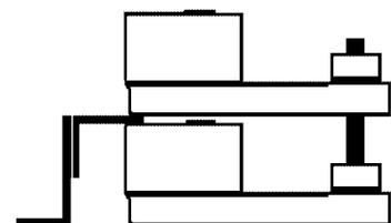
Note: The major advantage with this method is it requires less mounting area. The manual override, if available, cannot be used in this configuration.
