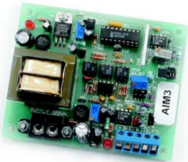
Analog Signal Isolation, 120 VAC Powered
