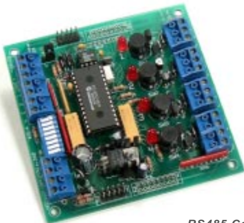
RS485 Controlled Lighting Contactor Interface
